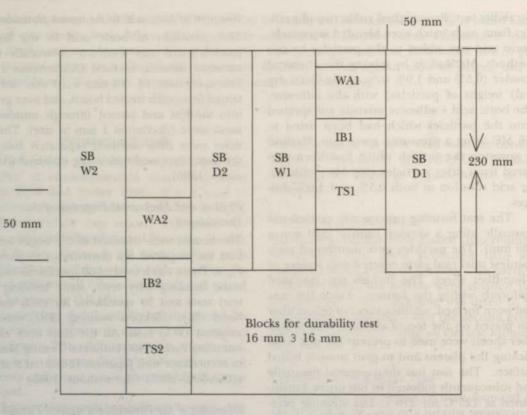
SBW = Wet static bending sample SBD = Dry static bending sample WA = Water absorption sample IB = Internal bond sample TS = Thickness swelling sample
